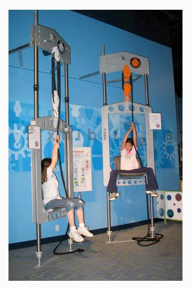
See how the mechanical advantage of rope and pulleys allow you to lift your own weight. The lift carriage can be raised up to 30" and is controlled to provide a slow, smooth descent. By choosing custom ratios of 3:1 and 6:1 children can experience their own weight on Mars or on the Moon respectively!
